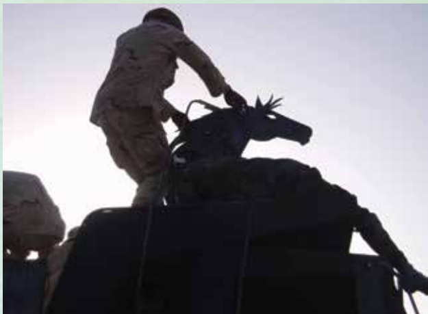
Spc. Rhett Crane welds a stallion's head made of half-inch steel in preparation for a convoy to Iraq from Kuwait in 2004. The "Iron Stallion" was mounted on top of a repurposed dump truck as a countermeasure for tripwires.
